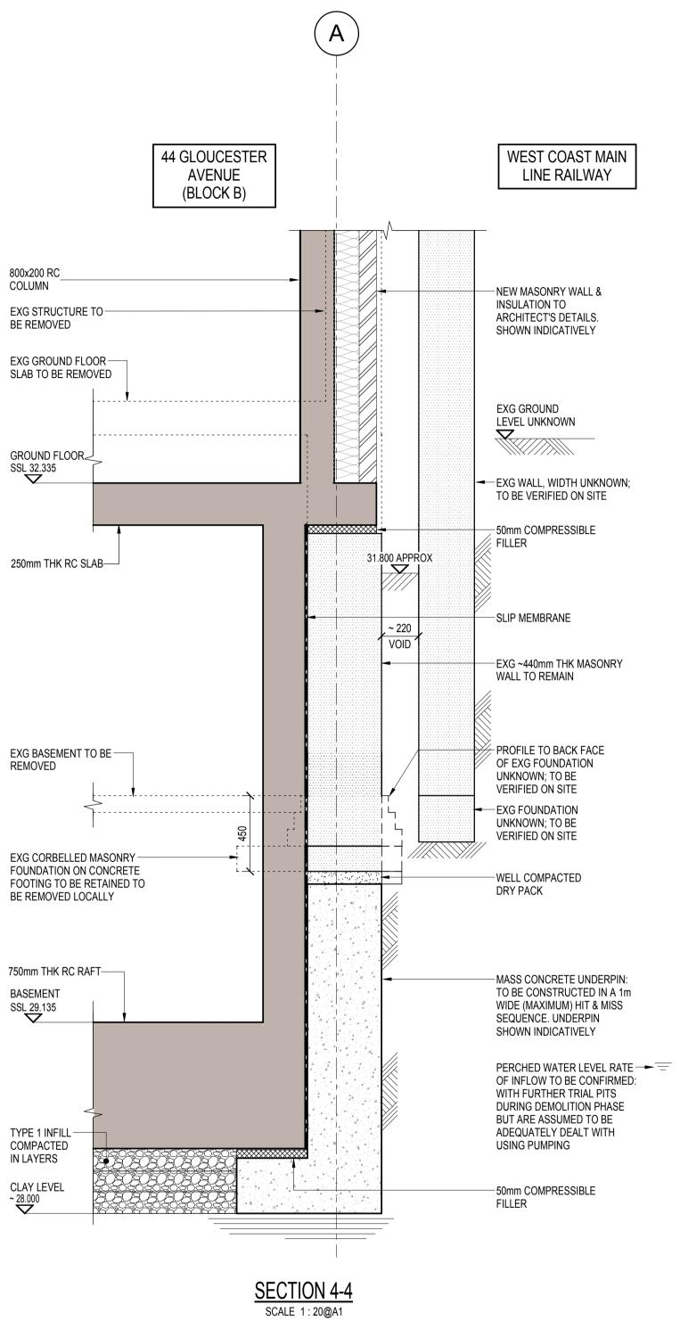
This drawing is to be read in conjunction with all relevant architects, engineers and specialists LEGEND drawings and specifications. Do not scale from this drawing. EXISTING STRUCTURE NEW MASS CONCRETE  $\equiv$   $\equiv$   $\equiv$   $\equiv$  LOAD BEARING STRUCTURE BELOW ----- EXISTING STRUCTURE TO BE REMOVED LOAD BEARING STUDWORK NEW LOAD BEARING BRICKWORK ------ NEW STEEL BEAMS NON LOAD BEARING WALLS NEW REINFORCED CONCRETE
