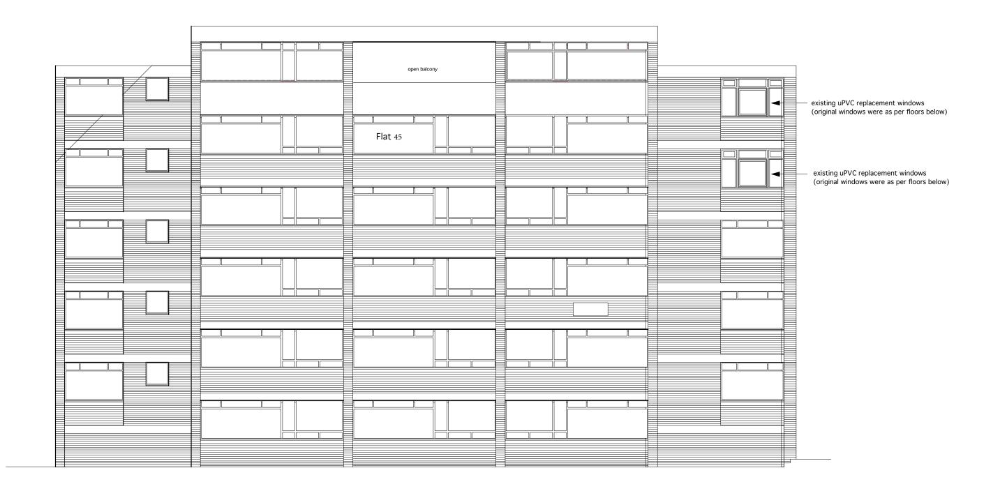
Existing Materials: Brick cross walls and brick panels between exposed floor concrete facias Concrete roof facias Concrete spandrel panels at 5th floor Tile hung spandrels ground to fourth Windows: brown painted hardwood single glazed
