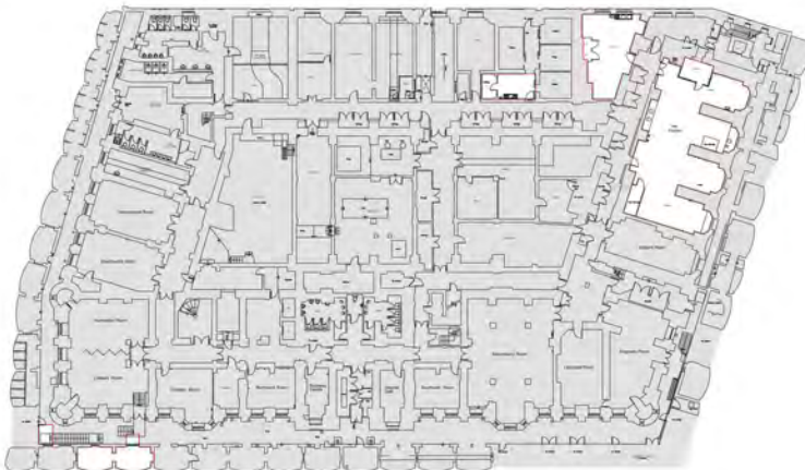
Proposed Lower Ground Floor Strip-out Plan - red outline denotes extent of lower ground floor contained within this planning application - blue hatching denotes extent of additional demolition contained within this planning application - red hatching denotes extent of demolition already approved within previous planning consent
