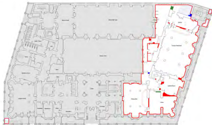
Proposed Ground Floor Strip-out Plan - red outline denotes extent of ground floor contained within this planning application - blue shade denotes extent of additional demolition contained within this planning application - red shade denotes extent of demolition already approved within previous planning consent
