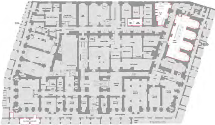
Proposed Lower Ground Floor Plan - red outline denotes extent of lower ground floor contained within this planning application - grey shade denotes extent of lower ground floor works consented under previous application and to remain unchanged
