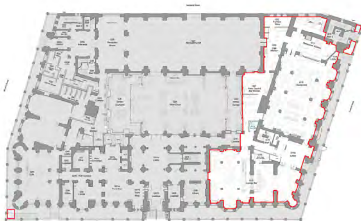
Proposed Ground Floor Plan - red outline denotes extent of ground floor contained within this planning application - grey shade denotes extent of ground floor works consented under previous application and to remain unchanged
