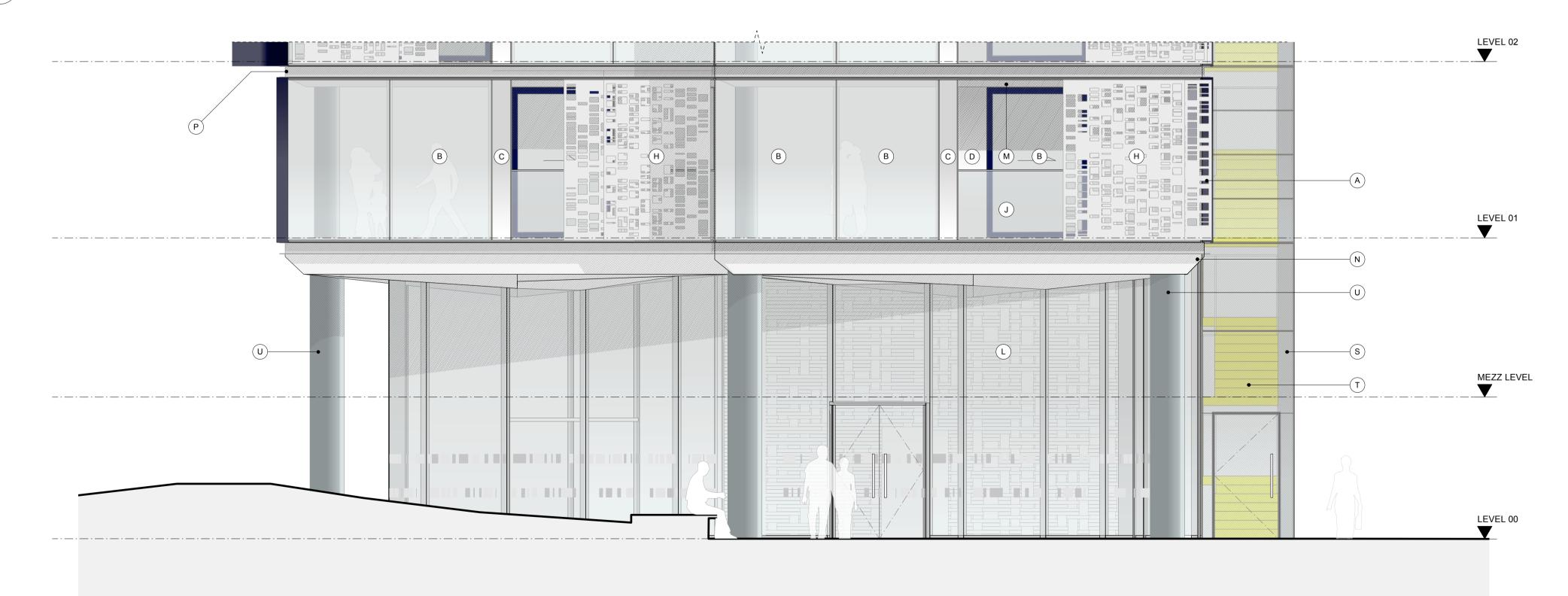
UNITISED FRAMELESS CURTAIN WALLING SYSTEM WITH CIRCA 200M DEEP GLASS RAINSCREEN FIXED TO OUTSIDE. RAL 5011 STEEL BLUE CERAMIC FRIT TO REAR (FACE 2) OF RAINSCREEN GLASS. GLASS REVEALS AROUND EDGES (TOP, SIDES AND SOFFITS) OF OVERALL RAINSCREEN ZONE TO MATCH
