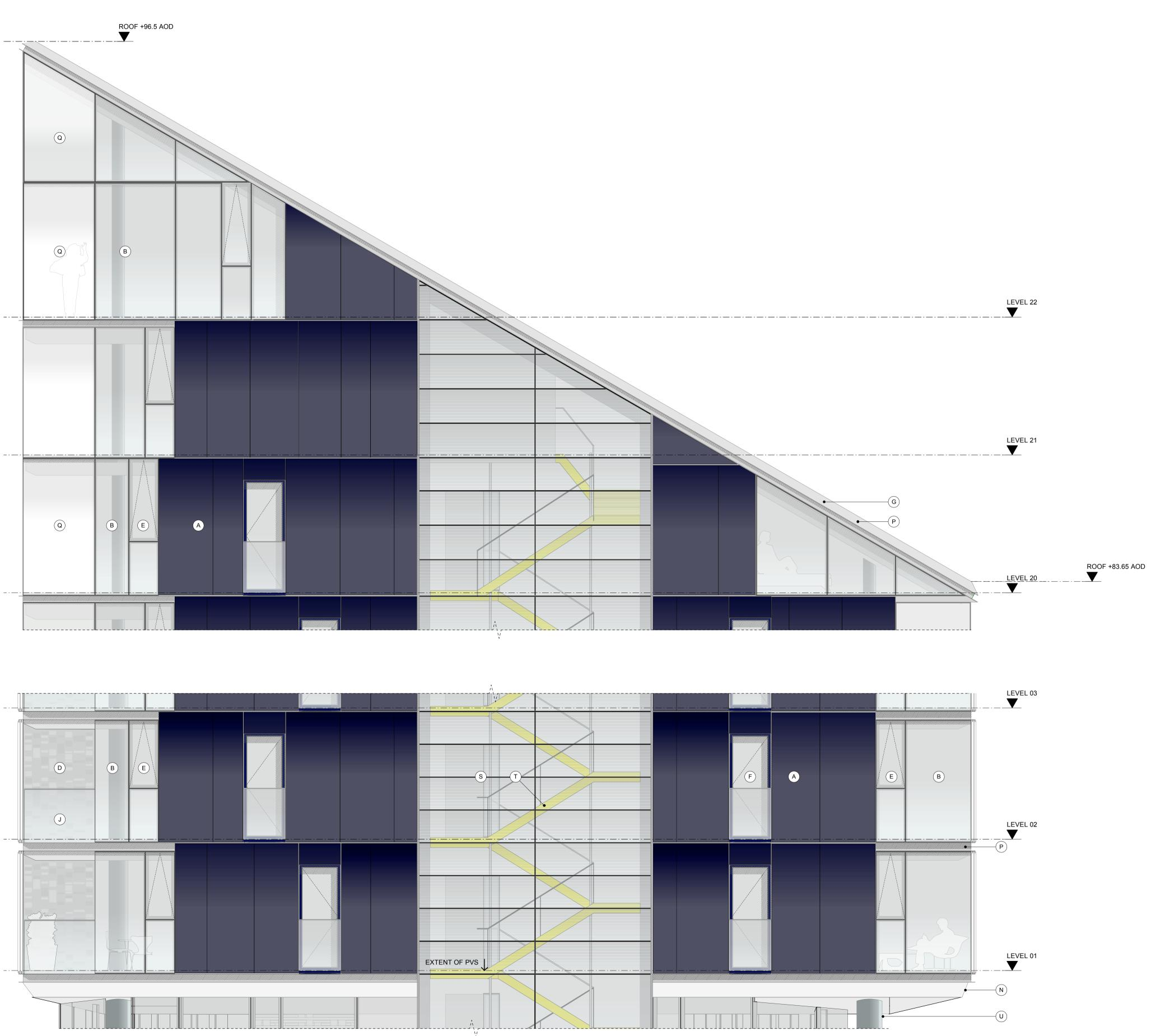
UNITISED FRAMELESS CURTAIN WALLING SYSTEM WITH CIRCA 200M DEEP GLASS RAINSCREEN FIXED TO OUTSIDE. RAL 5011 STEEL BLUE CERAMIC FRIT TO REAR (FACE 2) OF RAINSCREEN GLASS. GLASS REVEALS AROUND EDGES (TOP, SIDES AND SOFFITS) OF OVERALL RAINSCREEN ZONE TO MATCH
