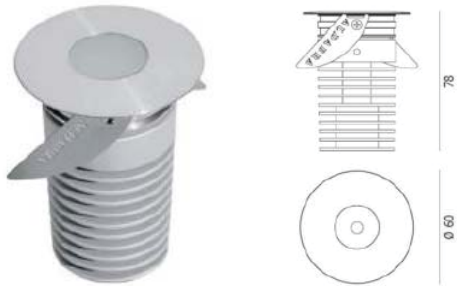
Recessed LED inground marker light, IP66 rated RGB, 4watts, R;12,32lm G;20,41lm B;4,87lm.
