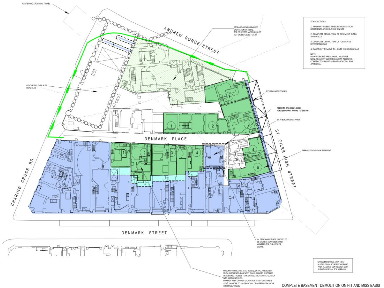
Figure 9.5.2: Breaking out of basements to be conducted in hit and miss arrangement.
