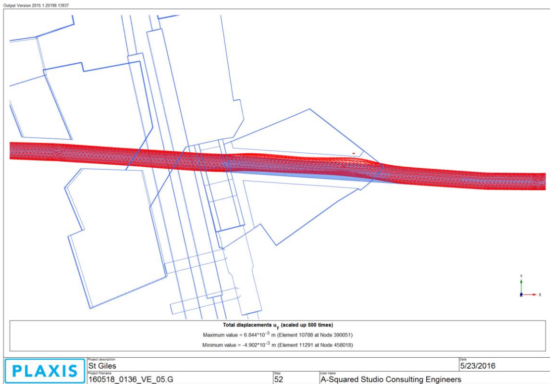
Figure 6.8: Short Term Crossrail tunnel deformation in horizontal plane.
