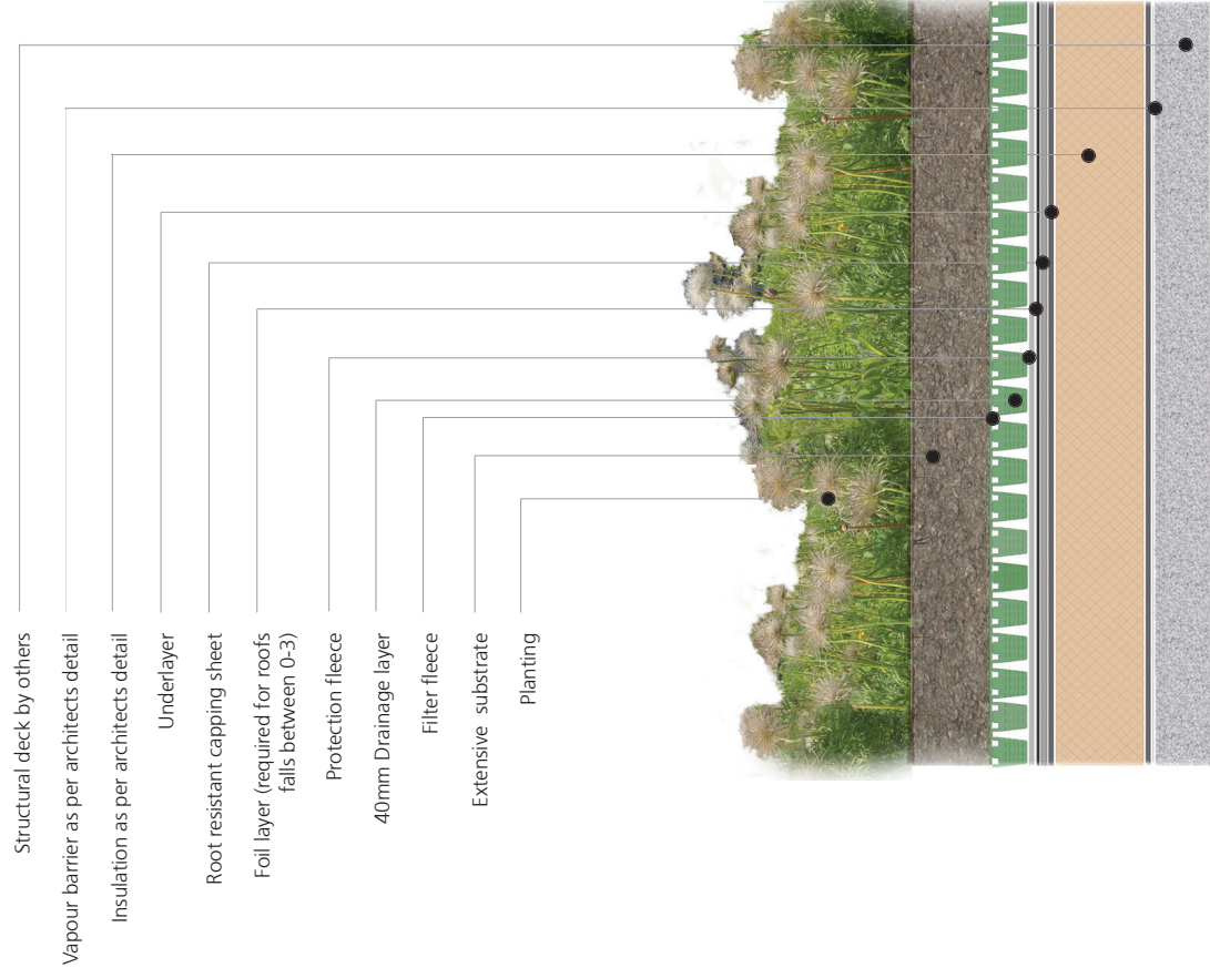
Extensive green roof section (scale 1:8)
