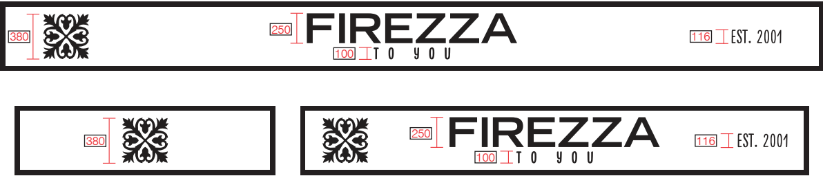
Proposed: Black letters with white halo illumination mounted to the existing a re-painted fascia. Internally illuminated projection sign.
