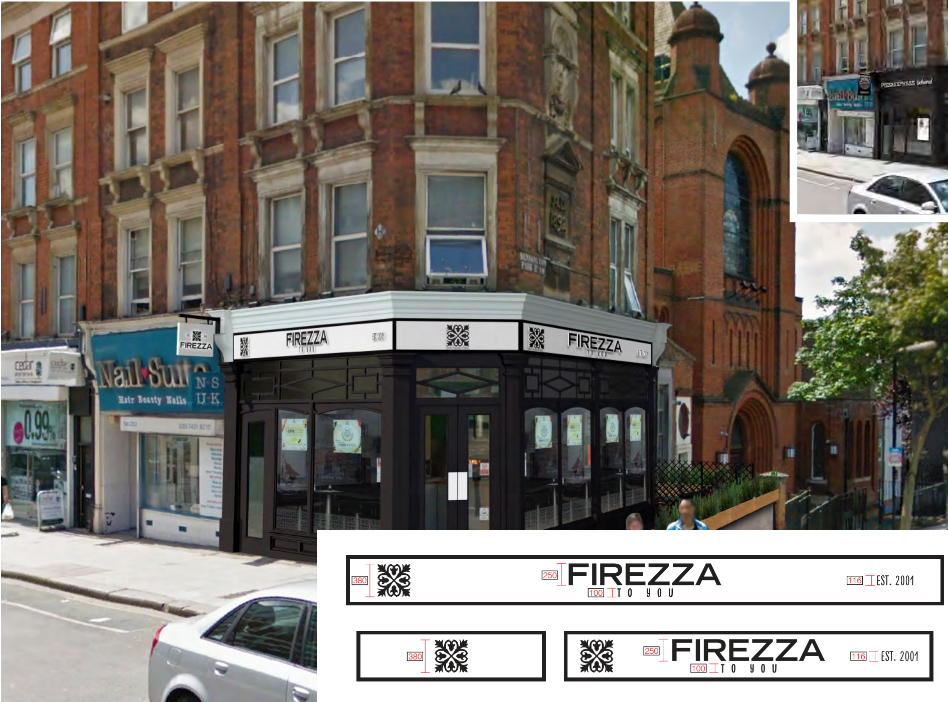
Proposed: Black letters with white halo illumination mounted to the existing a re-painted fascia. Internally illuminated projection sign.
