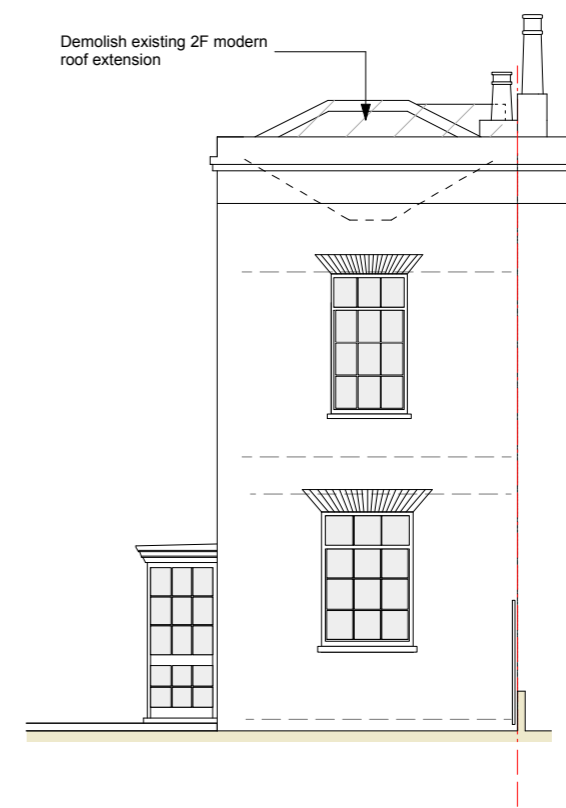
West Elevation : Existing Scale 1:100
