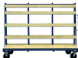
Large A-frame stillage Capacity 1000kg
