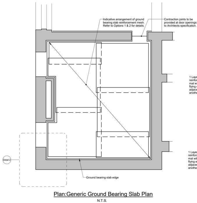
**Plan: Generic Ground Bearing Slab Plan**
