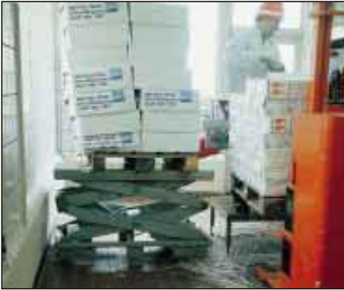
A 1 tonne capacity, hot dipped galvanised scissor lift in a food packing hall. Note how the base frame is raised to allow for relocation by fork truck.
