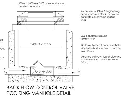
**BACK FLOW CONTROL VALVE PCC RING MANHOLE DETAIL**
