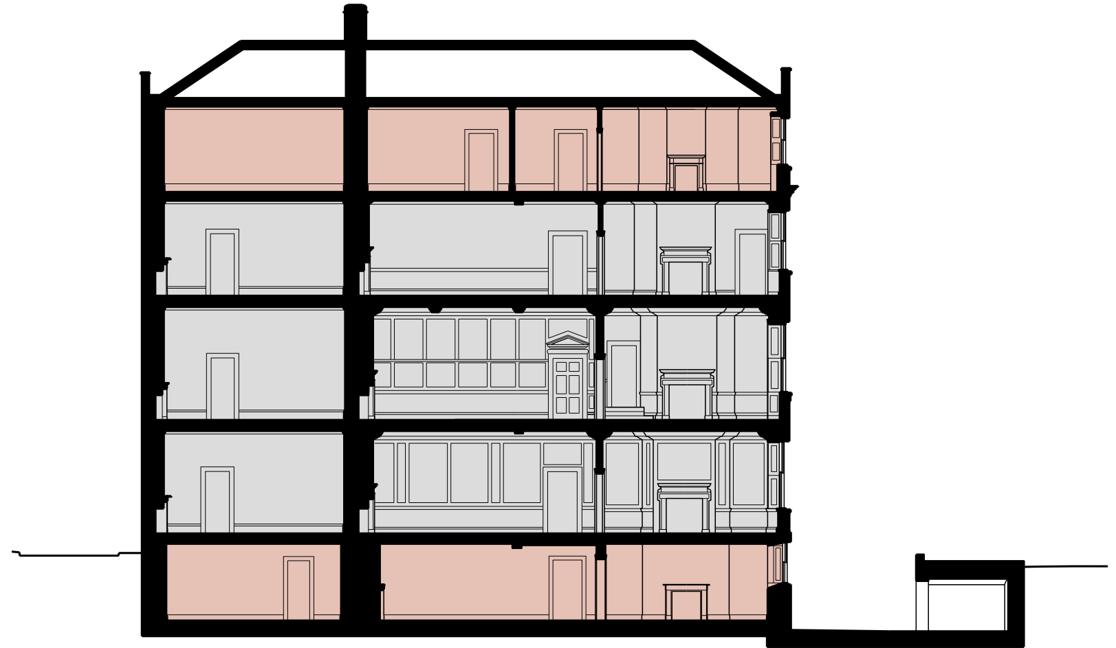
Section DD presenting areas of important historic fabric and areas for new architectural intervention.
