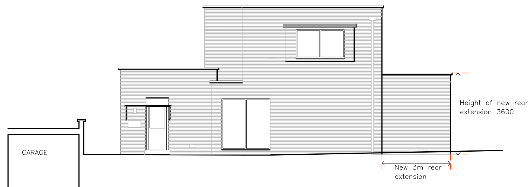
SECTION C-C (SIDE ELEVATION) AS PROPOSED 1:100@ A1
