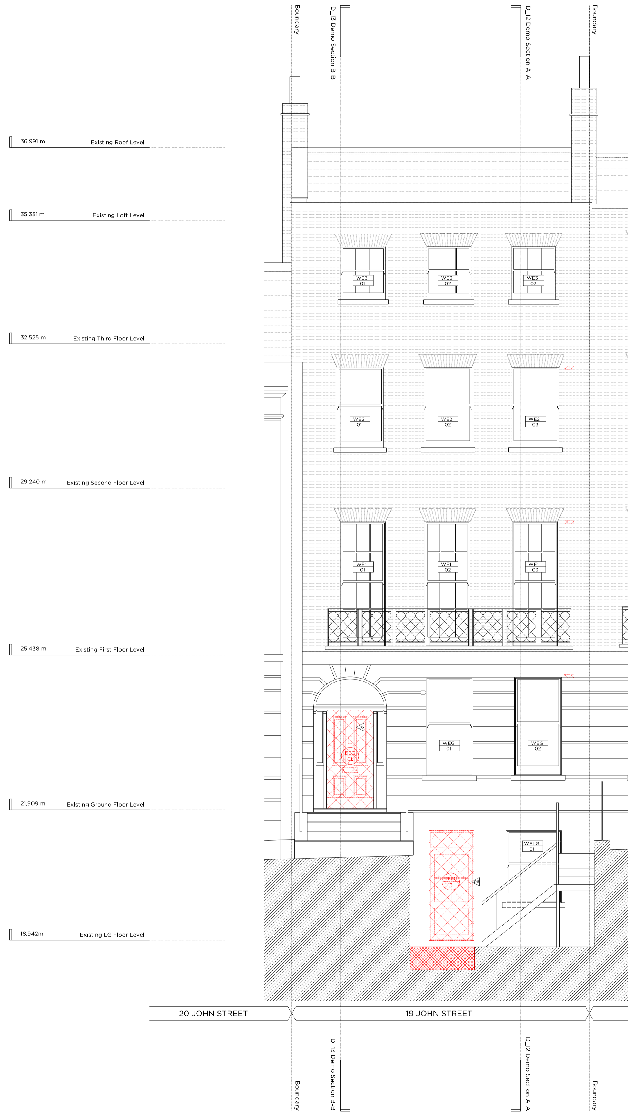
Demolition Front Lightwell Elevation
