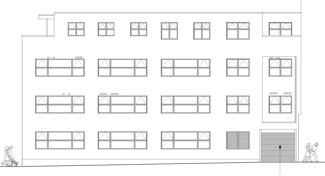
Existing painted metal roller shutter to be replaced with perforated painted metal shutter, for enhanced airflow to garage/ plant space
