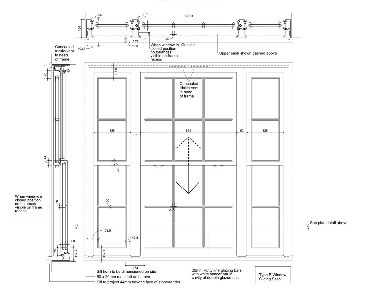
Do not scale from this drawing All dimensions to be checked on site - Double glazed units with white spacers bars and decorative astragal fixed over. Rev #. First Issue. 2016-07-20 Drawing type: L. B. CAMDEN Project: **LEVITA HOUSE PROPOSED** WINDOW TYPE B Scale: 1:10@A3 Date: 18/07/2016 Checked: SB Drawn: JMA Drg.no: 5675-A(31) TYPE B PROPOSED Rev: # Heritage Surveys Ltd. Heritage Surveys Limited 20 Hanover Square London W1S 1JY www.heritage-surveys.com
