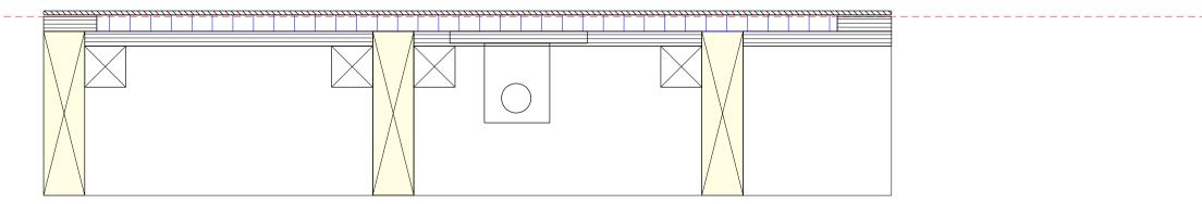
FLOOR DETAIL 02 New Shower floor buildup tiles on adhesive bed with ditramat debonding layer and electric heating mat Wetroom tanking system
