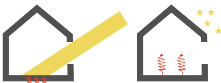
Examples of how the thermal mass absorbs heat during day and emits it during night.
