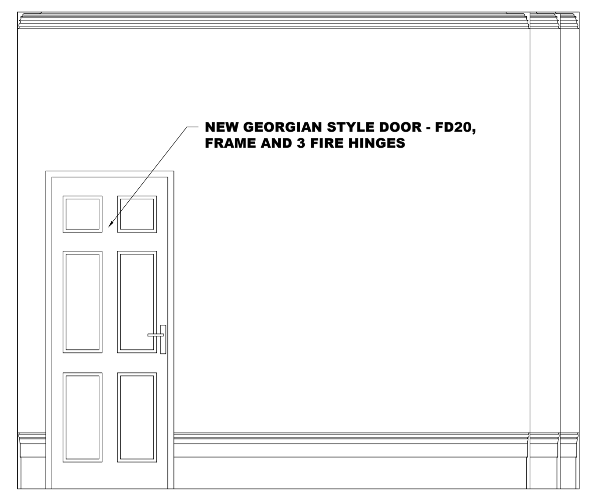
INTERNAL WALL ELEVATION VIEW 6
