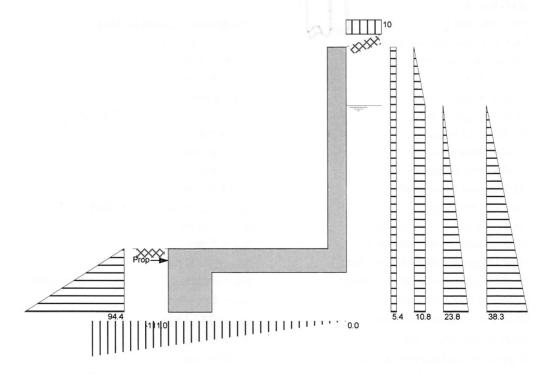
Loads shown in kN/m, pressures shown in kN/m<sup>2</sup>
