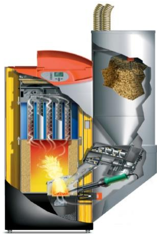
Figure 4.15: - Section through a Biomass Boiler
