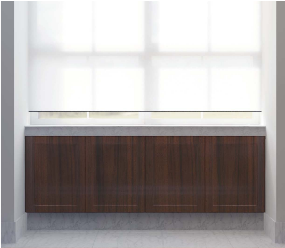
(above) Proposed new decorative timber boxing, with new marble skirting and concealed intake vent
