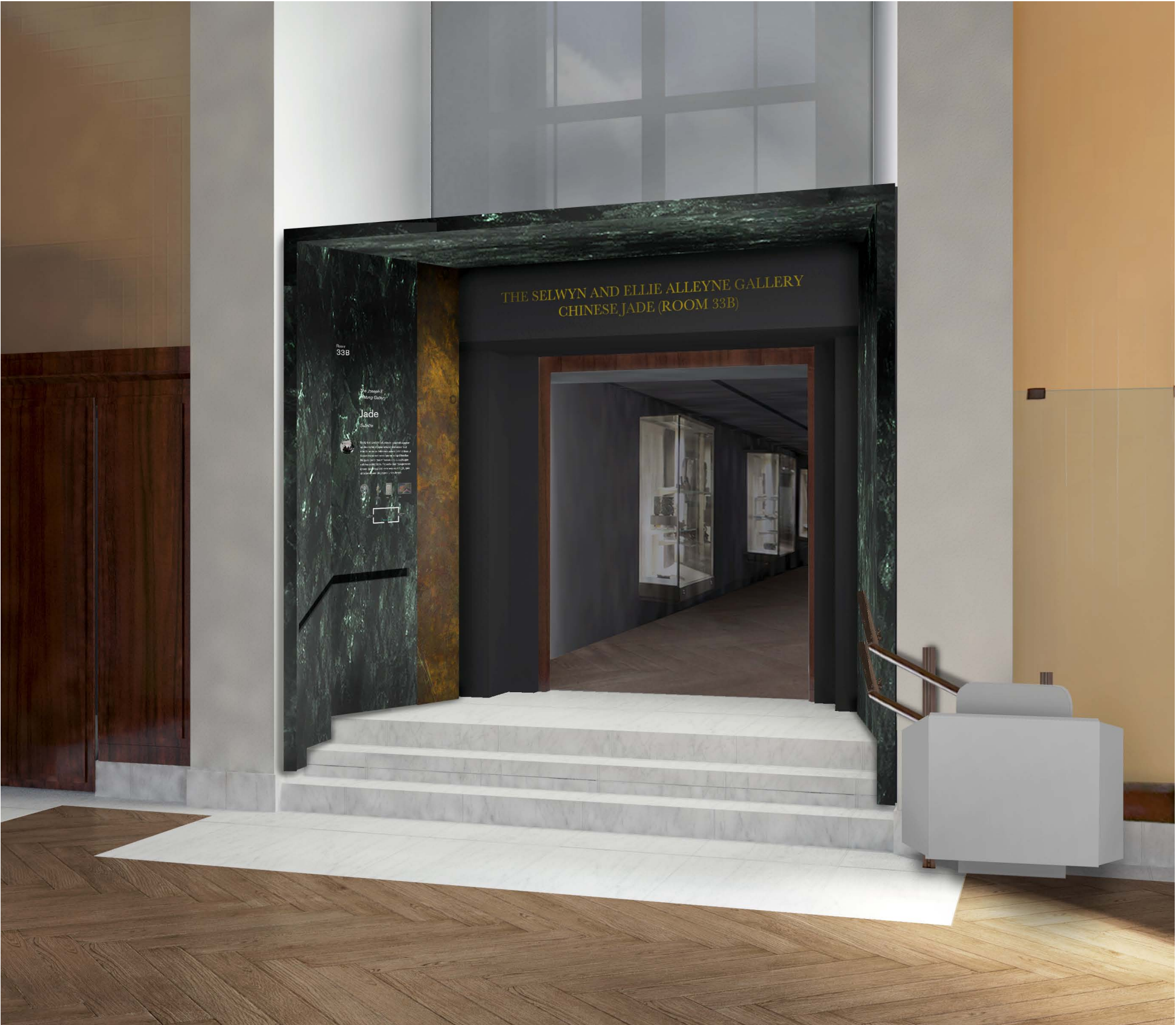
(above) Illustrative view of the proposed new 'portal' between Room 33 and Room 33b, with new discrete wheelchair accessible lift mounted on the right side
