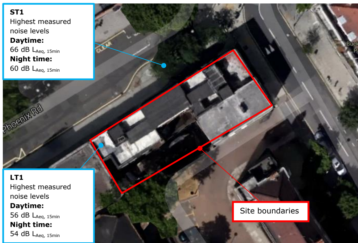
Figure 1: Site plan showing the measurement position and results of the highest measured L_{Aeq, 15min} noise levels.
