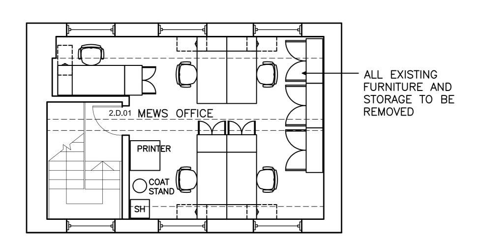
DOORS REMAINING AS EXISTING -2.D.01, 2.D.02, 2.D.03, 2.D.04, 2.D.05 (DOOR TO BE HANDED WITH NEW PARLIAMENT HINGES TO INCREASE DOOR SWING)
