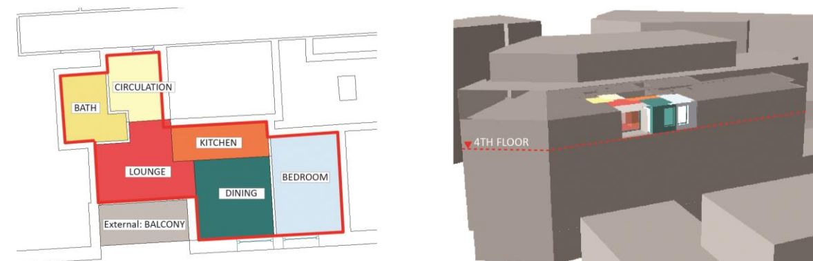
Figure 6: TAS EDSL model used for overheating risk assessment: zoning and 3d view.
