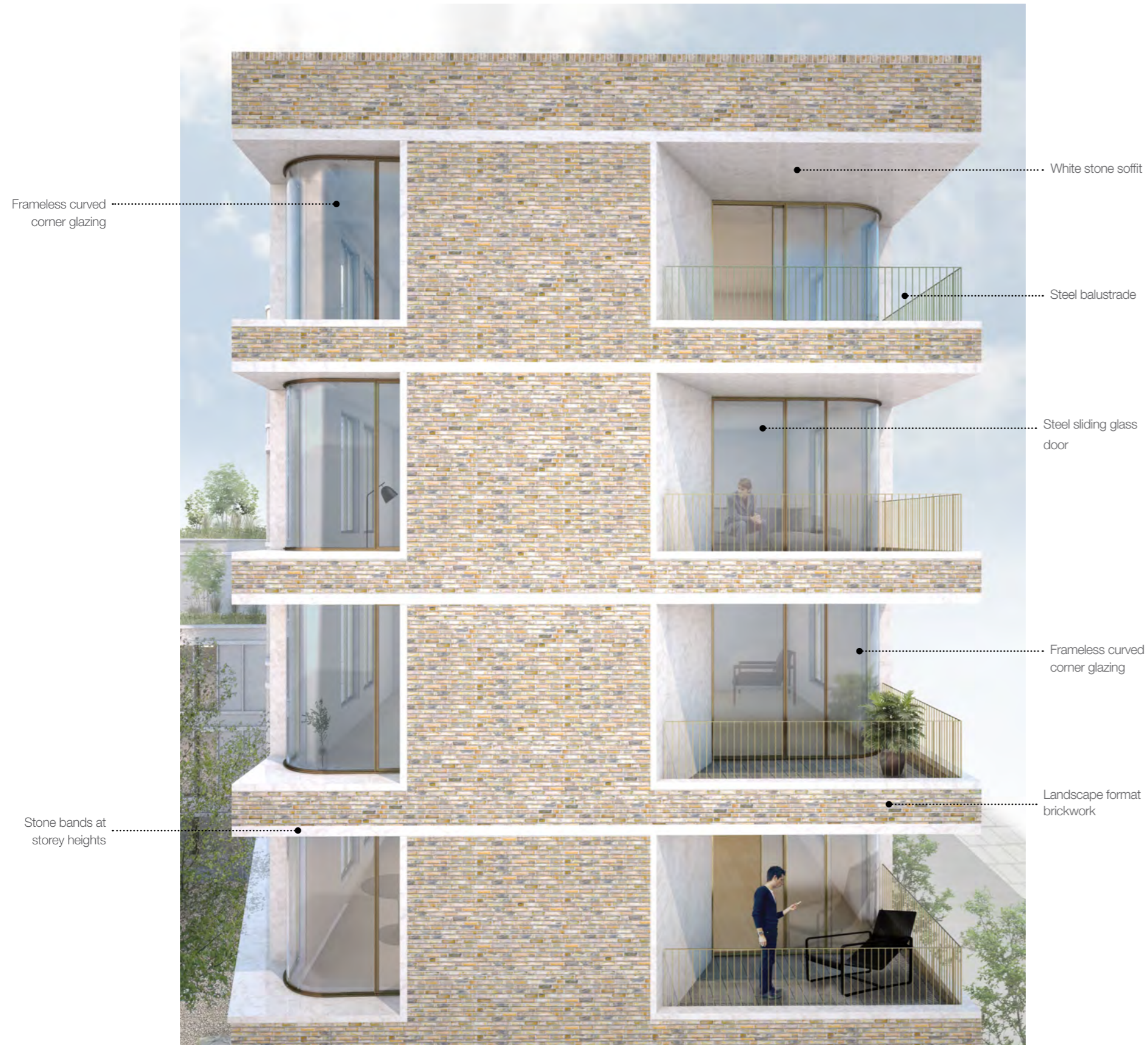
Corner Balconies and curved windows on gable end
