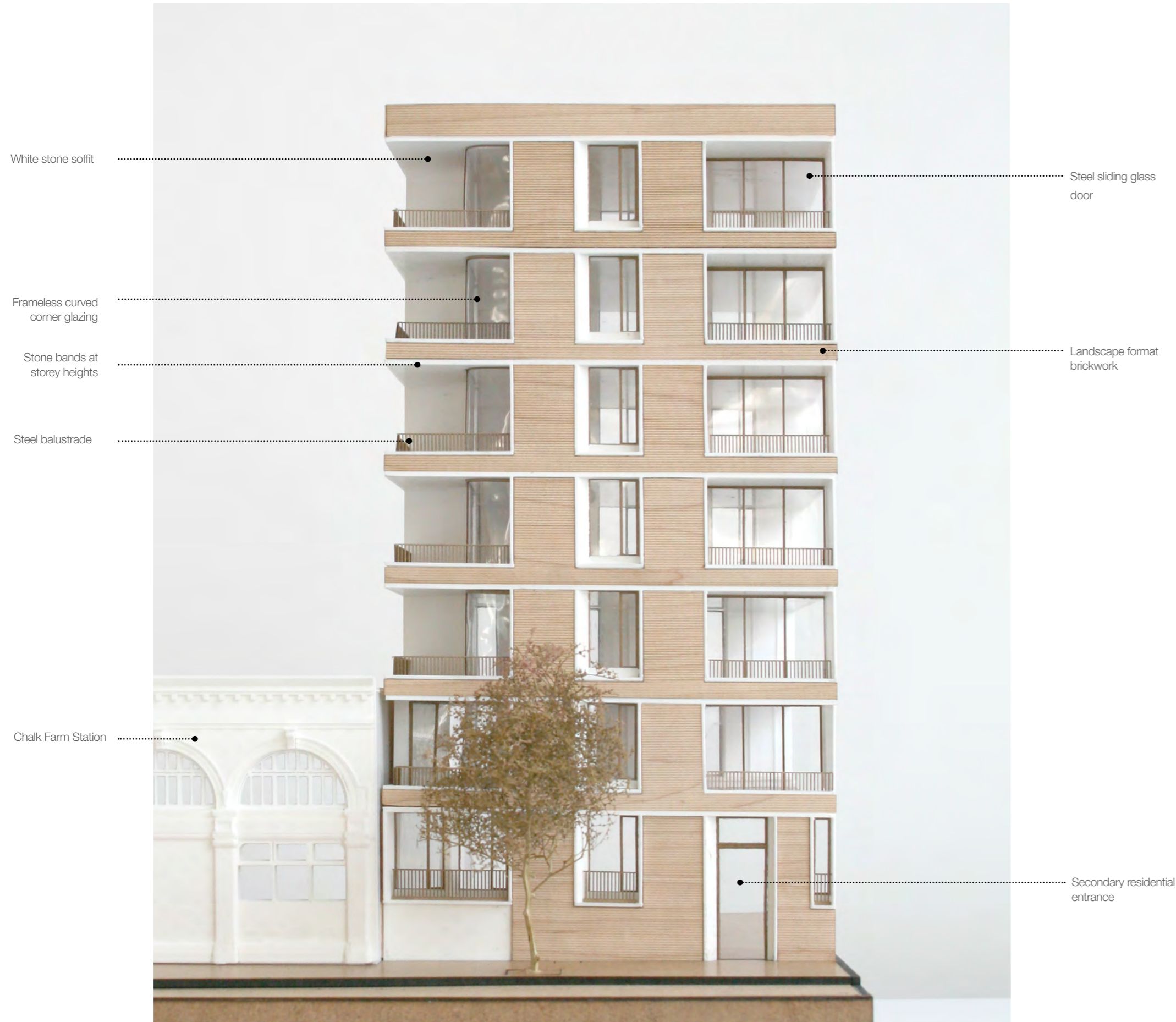
View of Haverstock Hill elevation next to Grade II Listed Chalk Farm Underground Station.
