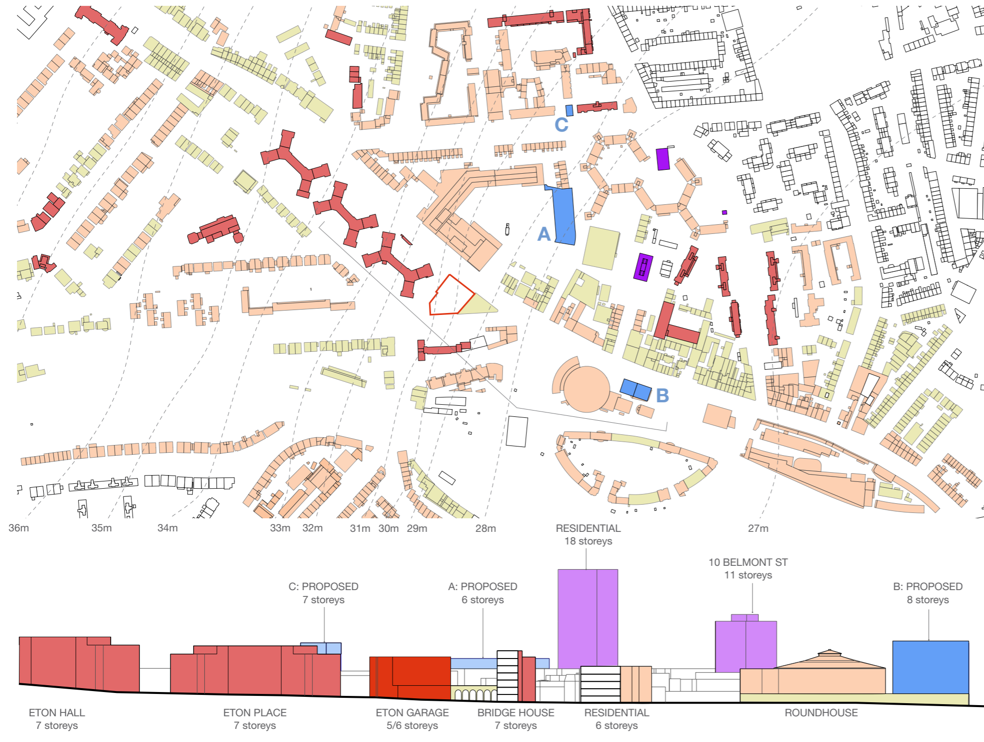
Site Plan and Section showing Building Heights
