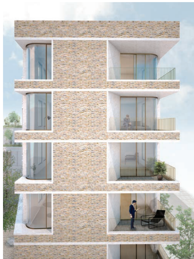
Fig. 5.2: Proposed corner balconies and curved windows on gable end.
