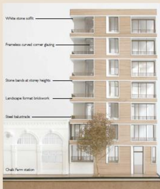
1:75 physical model of part of the Haverstock Hill Elevation
