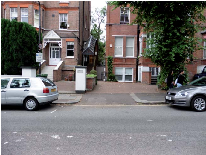
Figure 76. Two-car driveway with narrower crossover to right and left hand side of the tree (behind car). Gateway wider than crossover Note tall gate pier and mature garden tree (39 Netherhall Gardens).
