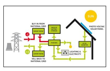
those that sit on top. Grid connected systems require very little maintenance, generally limited to ensuring that the panels are kept relatively clean and that shade from trees does not obstruct the sunlight path. However, the wiring and system components should be checked regularly by a qualified technician.
