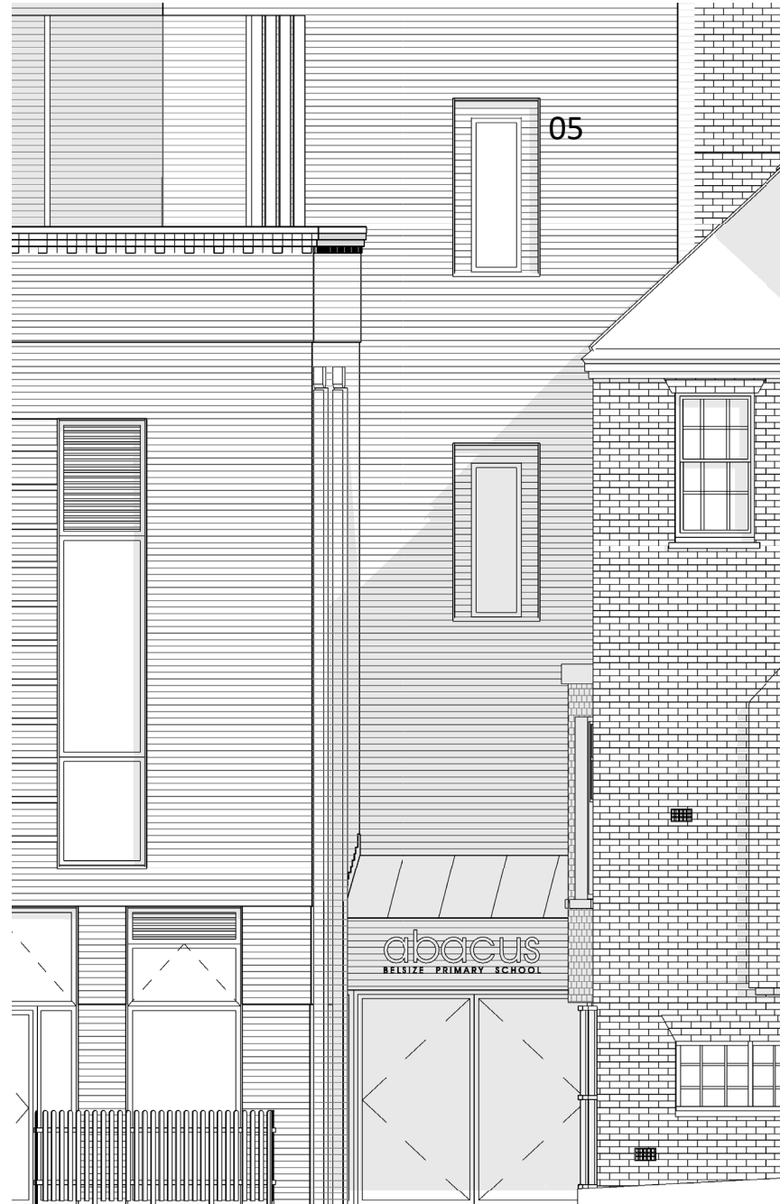
Extract from Rear Elevation showing windows with trim only and windows to the staircase with trim and margin. (Not to Scale)
