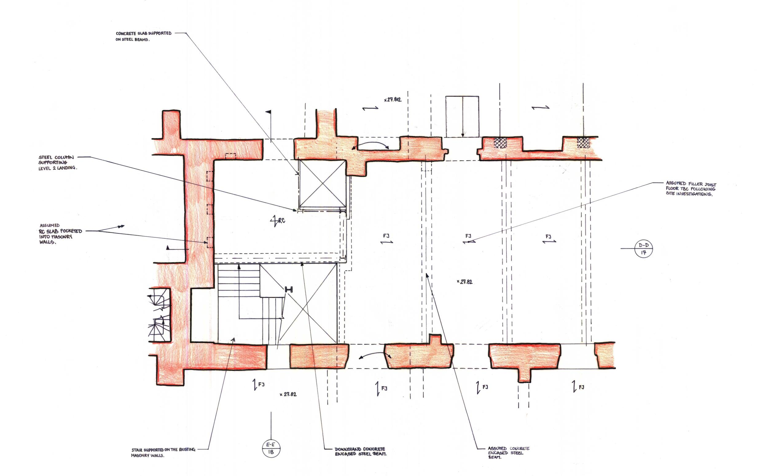
1. THIS DRAWING IS TO BE READ IN CONJUNCTION WITH ALL RELEVANT ARCHITECTS AND ENGINEERS DRAWINGS AND THE SPECIFICATION. 10.5.16 ISSUED FOR DISCUSSION . **BRITISH MUSEUM** WHITE WING **CRAWFORD STAIR** EXISTING STRUCTURE LEVEL 02 PLAN scale (original - A1)
