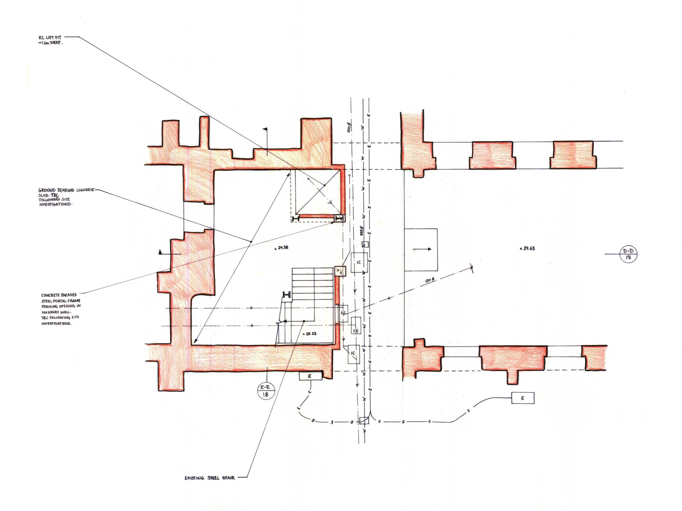
I. This drawing is to be read in conjunction with all relevant architects & Engineers drawings & the specification. 2. KEY: EXISTING DRAINAGE E EXISTING ELECTRIC EXISTING INSPECTION CHAMBER ELECTRIC DISTRIBUTION
