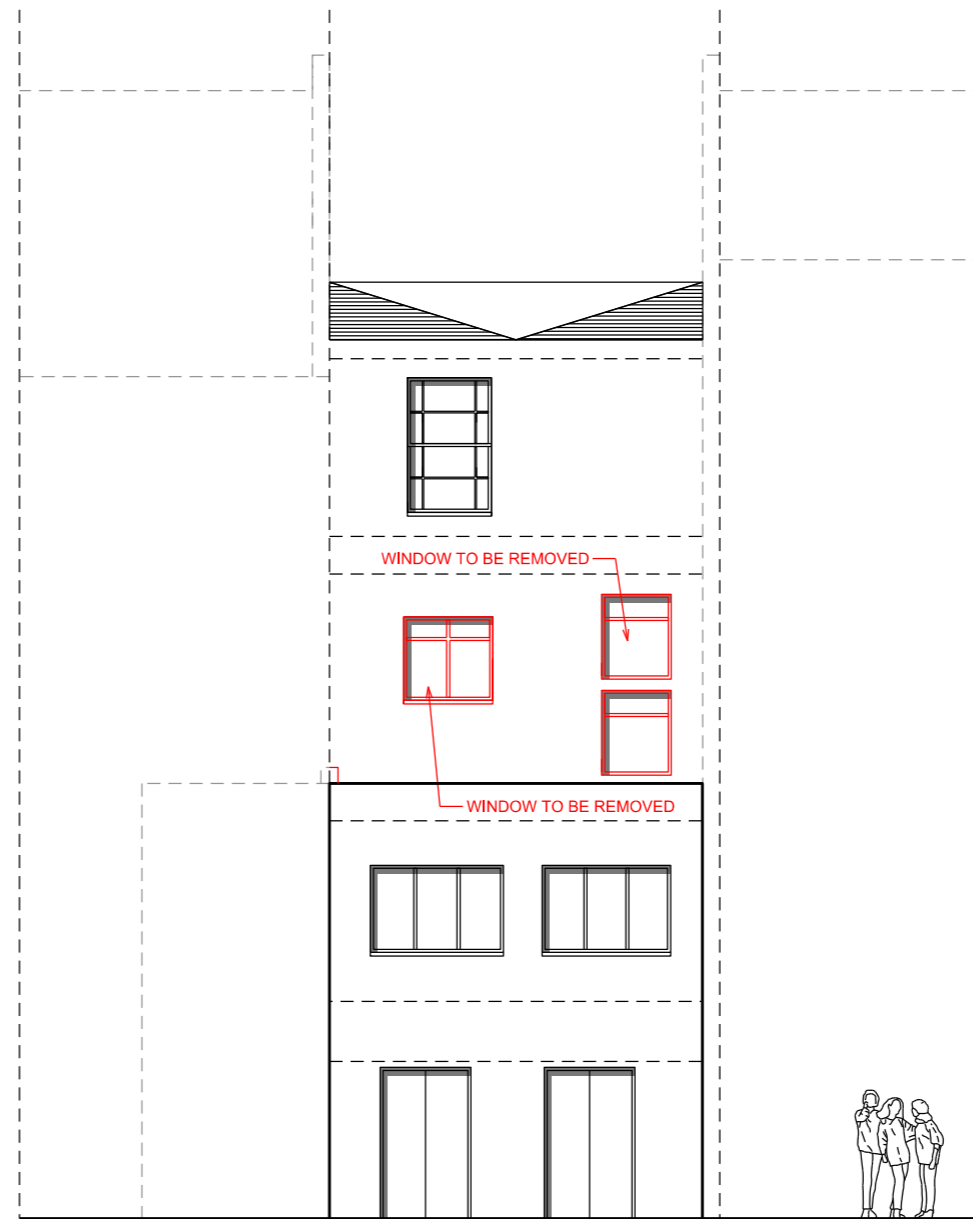
② EXISTING / DEMOLITION REAR ELEVATION
