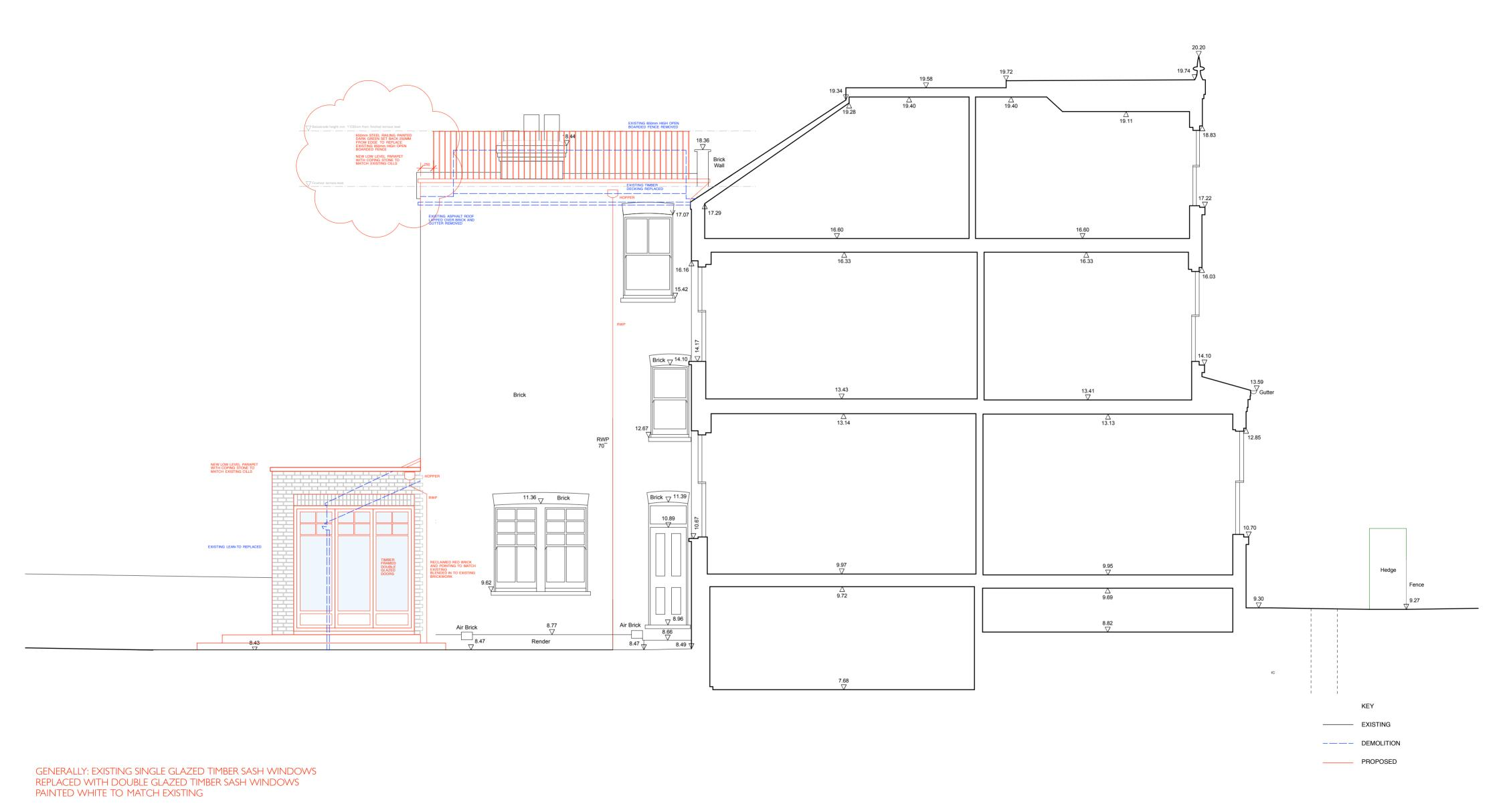
Rev A - 08/09/2015 - GLAZED BALUSTRADE ALTERED TO SIMPLE BLACK RAILINGS AS ADVISED BY CASE OFFICER Rev B - 01/10/2015 - FIRST FLOOR TERRACE REMOVED, RAILINGS TO THIRD FLOOR TERRACE REDUCED IN HEIGHT AND SET BACK FROM EDGE Rev C - 08/07/2016 - THIRD FLOOR ROOF TERRACE RAILING COLOUR AMENDED scale 1:50@A2 date AUG 2015
