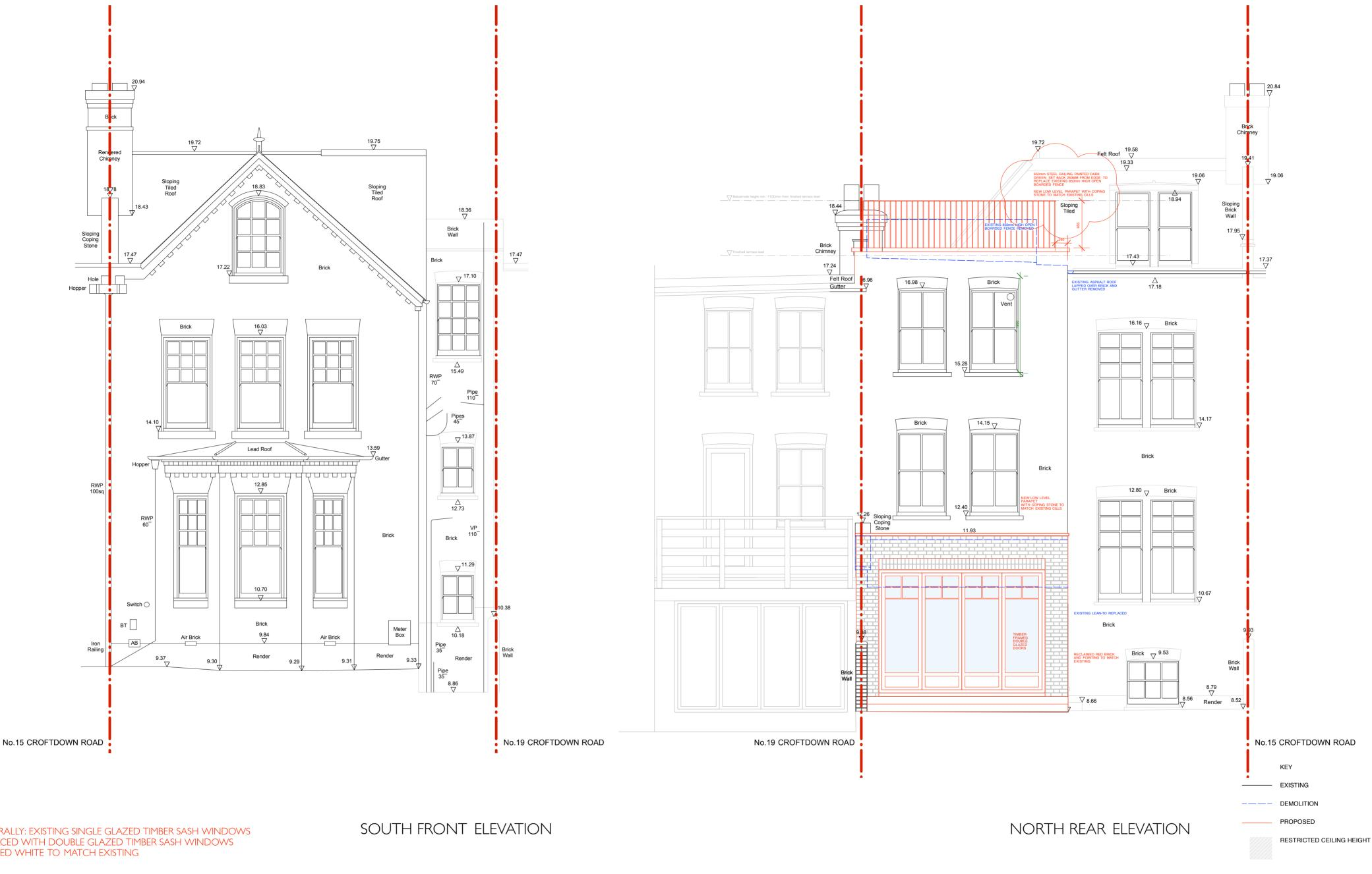
GENERALLY: EXISTING SINGLE GLAZED TIMBER SASH WINDOWS REPLACED WITH DOUBLE GLAZED TIMBER SASH WINDOWS PAINTED WHITE TO MATCH EXISTING
