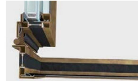
OS2 outward opening window is an integrated system with accessories, seals and thermal break profiles 65 mm deep allowing for a wide range of windows, rectangular, shaped or curved. They can be equipped with double glazing up to 30 mm thick. Each solution is equipped with a related set of accessories integrated in the system.
