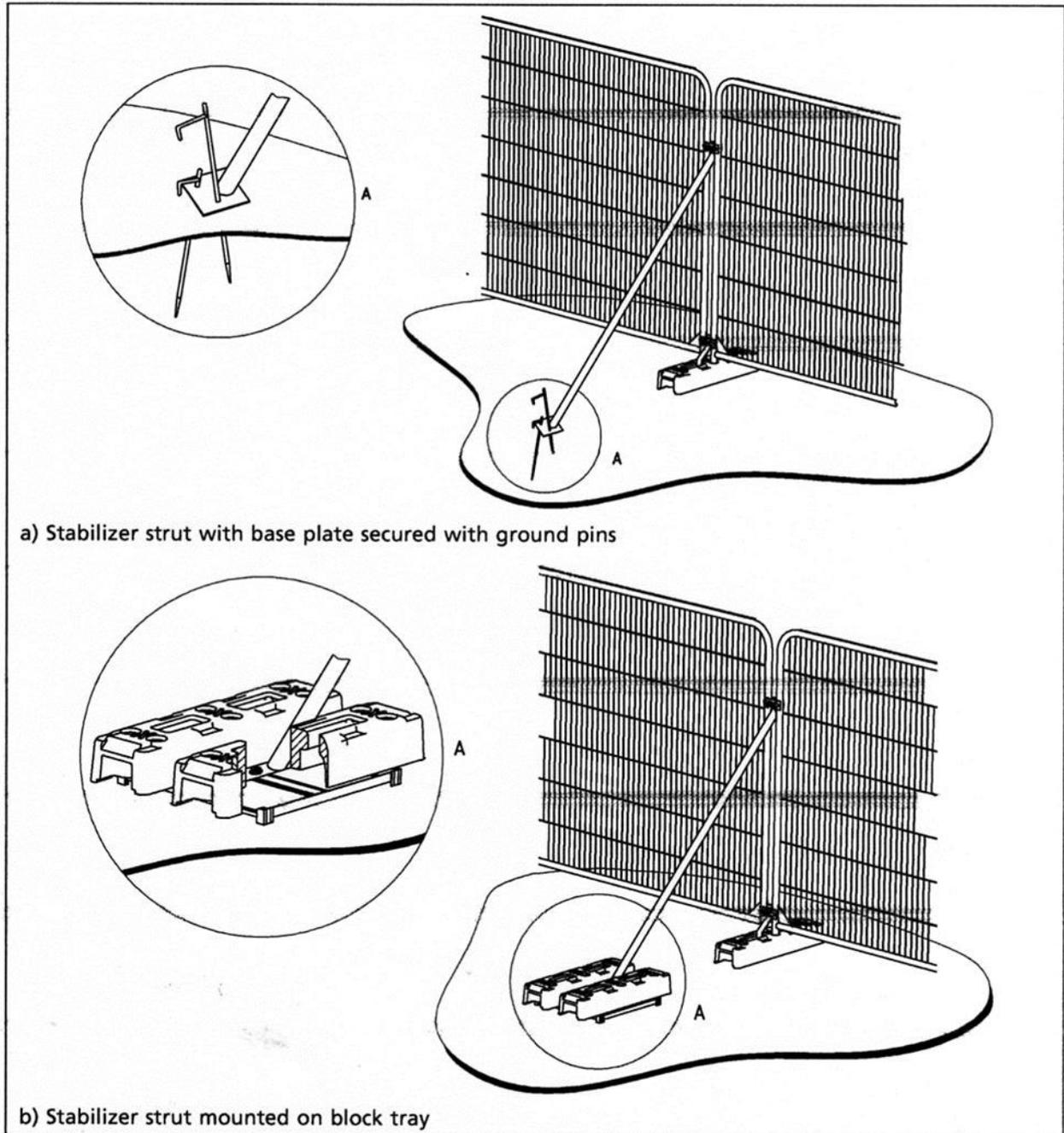
a) Stabilizer strut with base plate secured with ground pins
