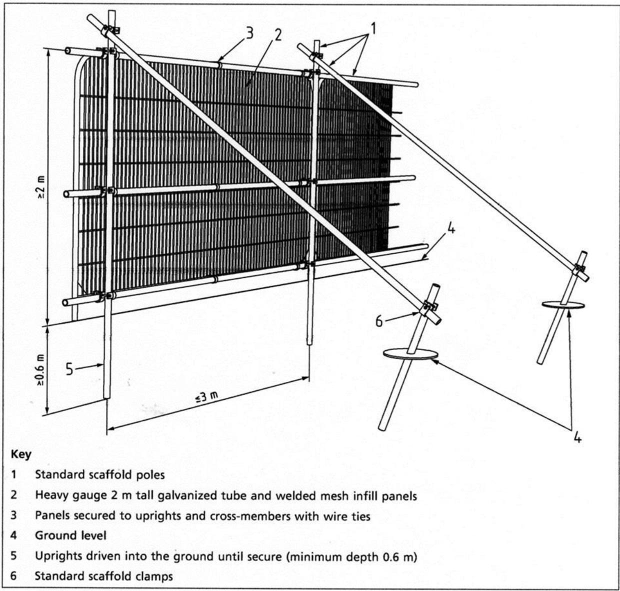
Figure 3 Examples of above-ground stabilizing systems
