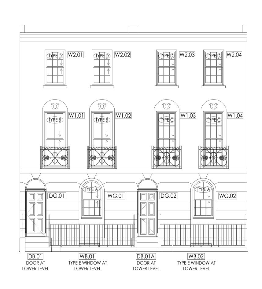
PROPOSED FRONT ELEVATION SCALE 1:50 @ A1
