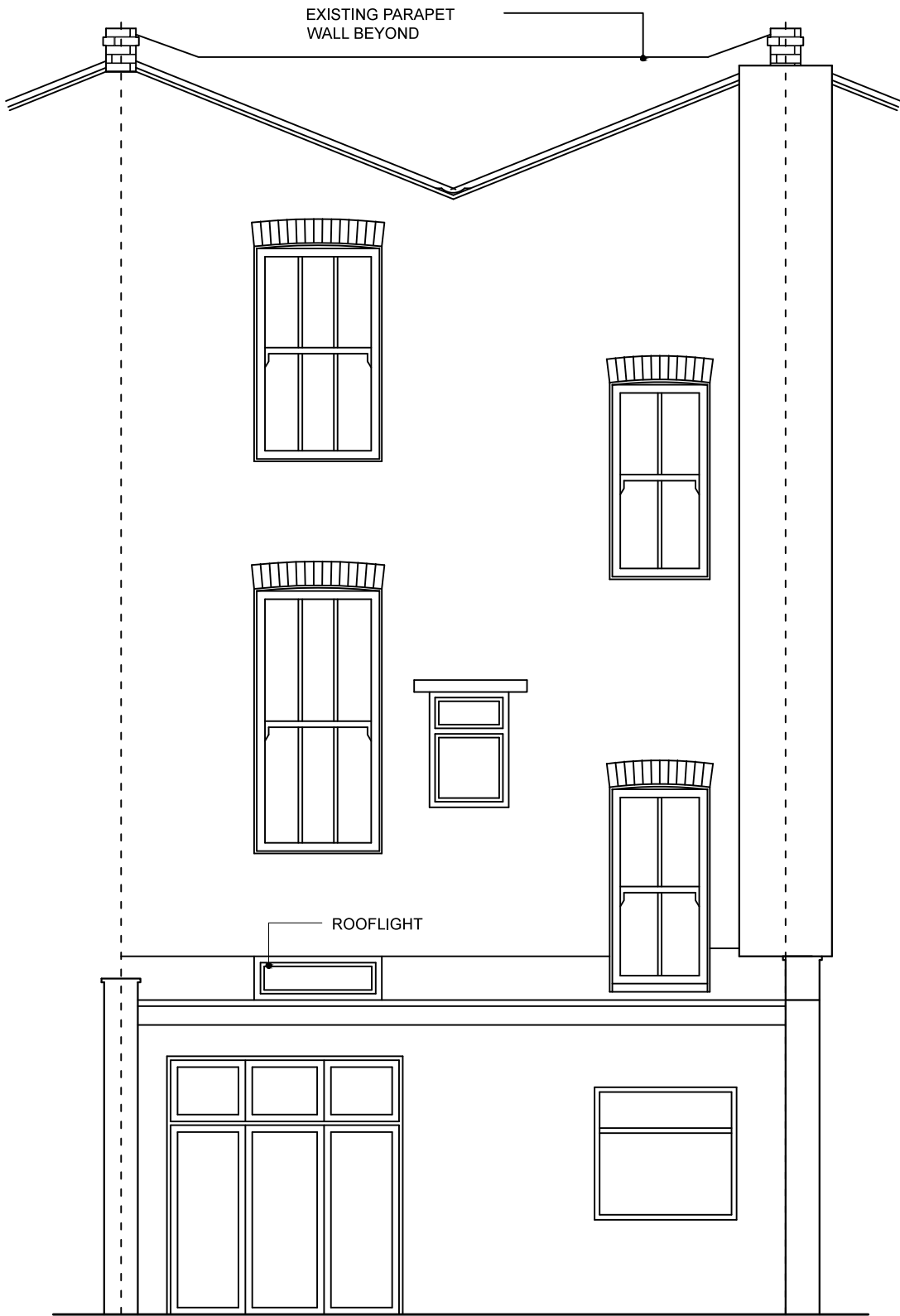
EXISTING REAR ELEVATION
