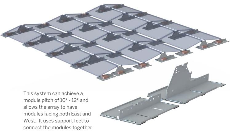
throughout the array. It uses the principle of aerodynamics to create suction underneath the system, therefore reducing the amount of additional ballast required to keep the array in place.
