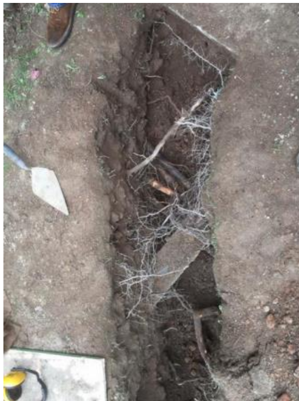
Photograph 3: Packet of significant roots found (2 x 45mm, 1 x 40mm diameter)
