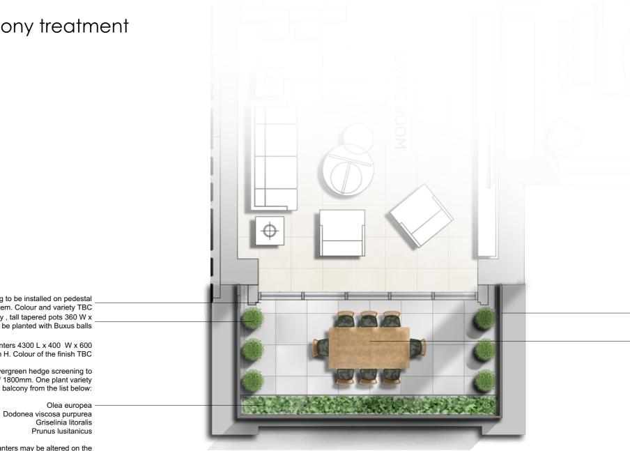
Porcelain paving to be installed on pedestal system. Colour and variety TBC High quality clay, tall tapered pots 360 W x 1000 mm W. To be planted with Buxus balls
